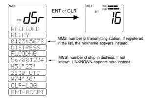
The displayed message continues until either ENT or CLR is pressed. At that time, the radio switches to Channel 16 in high power and the contents of the communication are stored in the Log File.
